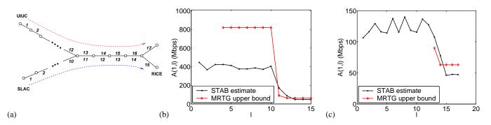
**Figure 3:** (a) Experiment topology. Available bandwidth from the sender to intermediate hops l, A(1, l), for path (b) SLAC–Rice and (c) UIUC–Rice measured from a 1 hour interval.
