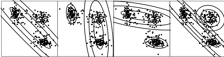
Figure 2: Several L2E mixture fits to the lagged Old Faithful geyser eruption data with K = 1 and K = 2 ; see text. The weights in each frame are (1.0) , (.258, .742) , (.714, .286) , and (.711, .289) .
