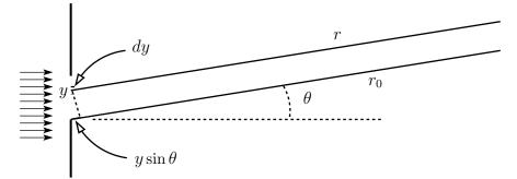
Call the coordinate along the width of the slit y, where 0 < y < a. I want to find the total light wave that passes through the slit and that heads at the angle  $\theta$  away from straight ahead. The light that passes through between coordinates y and y + dy is a wave
